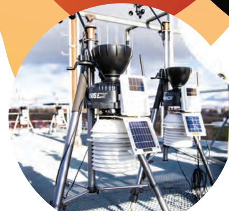
A rooftop meteorological station, high above the TUM School of Life Sciences Campus, is used for measurements and for testing measurement equipment before field use.
